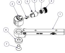
Figure 3: Exploded diagram of CNC-lathe version GW520-16U
